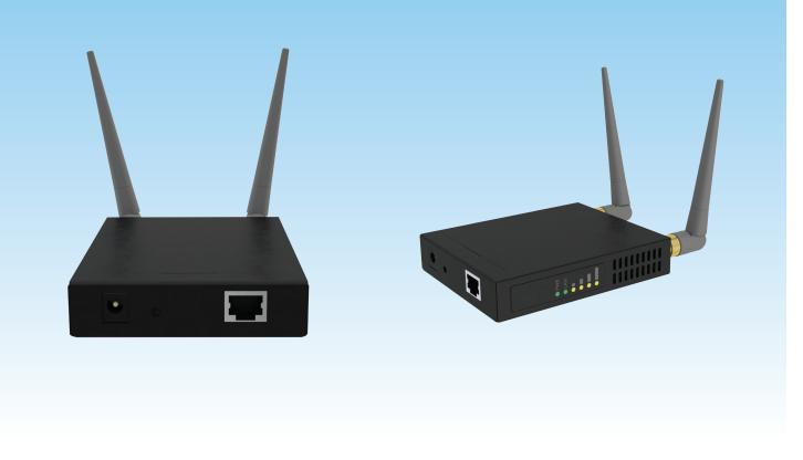
The APC 5Mi is a small, but robust and high performance 5 GHz access point designed for indoor applications. This product is equipped with an extreme output power (up to 29 dBm) 802.11n MIMO radio which allows communicating effectively older 802.11b/g equipment together with latest standards wireless devices. The APC 5Mi is coupled with an advanced and feature-rich operating system which allows the product to operate as an access point and as a station at the same time,
